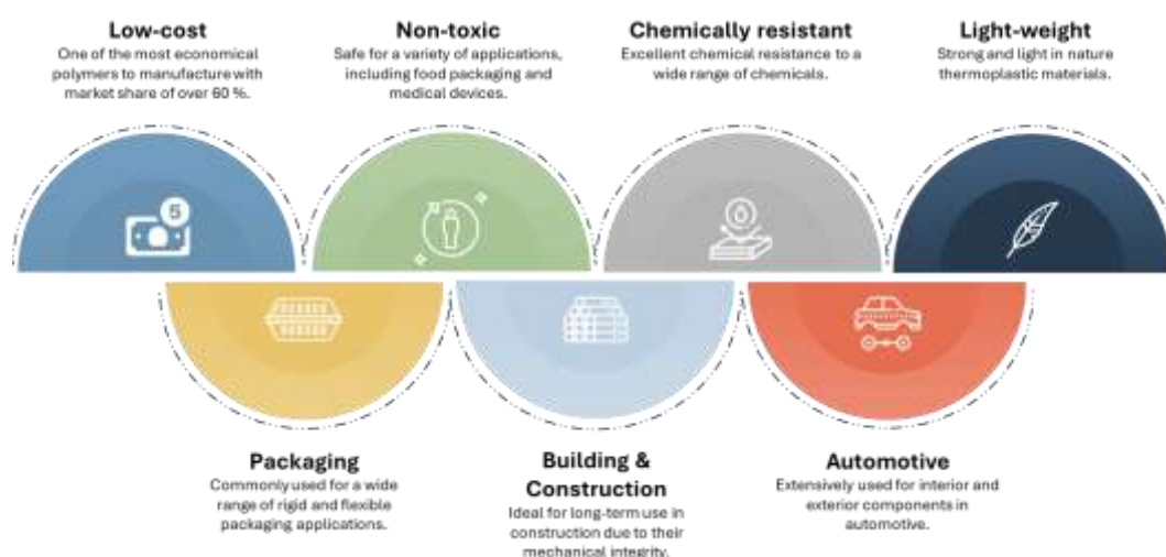
Figure 1.3. Primary characteristics and major industrial applications of commodity polyolefins. 9
