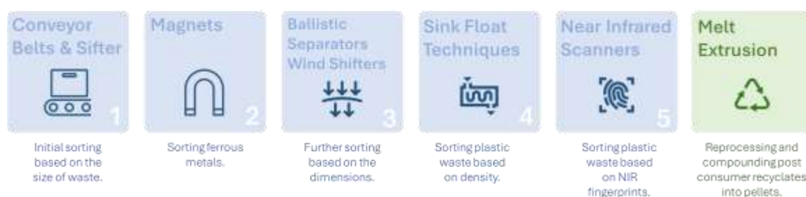
Figure 1.7. Industrial workflow for the sorting and mechanical recycling of post-consumer plastic waste.
